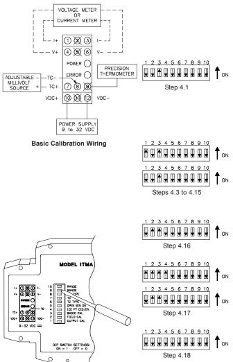
Note: The nominal output value for the various output ranges are designated in the following order: (0 to 20 mA, 4 to 20 mA, 0 to 10 VDC)
