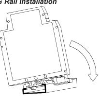
To install the ITMA on a "T" style rail, angle the module so that the top groove of the "foot" is located over the lip of the top rail. Push the module toward the rail until it snaps into place. To remove a module from the rail, insert a screwdriver into the slot on the bottom of the "foot", and pry upwards on the module until it releases from the rail.
