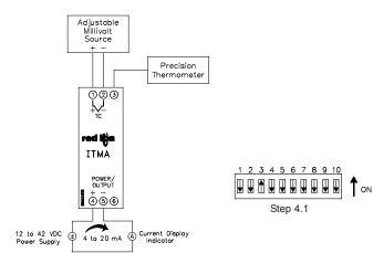
Basic Calibration Wiring
