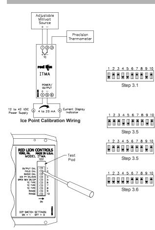
The Ice Point Calibration should only be performed with an ambient temperature between 21°C and 29°C. This Calibration was performed on the unit at the factory during the Basic Calibration and generally does not need to be done again. The Ice Point Compensation can be adjusted through this calibration. The Ice Point Calibration procedure is described below.
