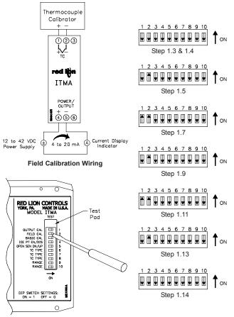
Field Calibration scales the 4 to 20 mA output to a temperature or mV input. This procedure assigns an input value to 4 mA and an input value to 20 mA. The microprocessor handles configuring the output so it is linear to the temperature or mV input. The Field Calibration procedure is described below.
