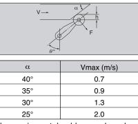
The maximum tolerable speed can be extended by further reducing the dog rise angle from 45° when 0.5m/s <  $V \leq 2m/s$ . It is necessary to set the arm so that the dog's cutting surfaces are always parallel ( $\theta \circ = 90^\circ - \alpha$ )
