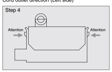
Confirm the fitting metal is on tightly. If it is loosen, it might be cause of the trouble.
