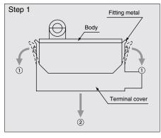
Push down the fitting metal while pulling it horizontal direction.
