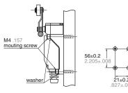
Depth of screw holes > 15mm .591inch
