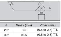
Even if overriding the dog, set the forwards and rearwards motion exactly the same, and avoid any settings that make the actuator accelerate rapidly from the dog.
