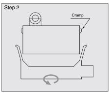
Turn the terminal cover at an angle of 180 degree. Follow the procedure 3.
