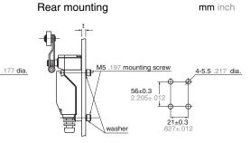
Length of bolt < panel thickness t+7mm .276inch
