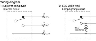
Note: Since LED is connected to N.O. side, the polarity of the load shall be + for N.O.
