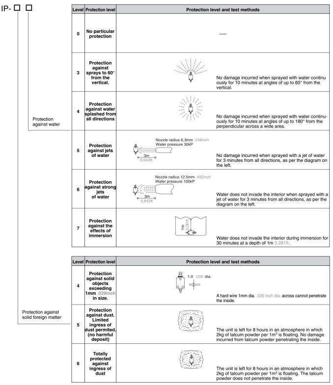
Notes: 1. All of the tests cited above were conducted with the cord vent (conduit vent) tightly shut.
