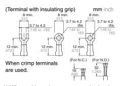
8) When wiring, do not connect the lead wires directly to the terminals, but use the crimp terminals and tighten them to a torque of 0.39 to 0.59 N•m {4 to 6 kg·cm}.
