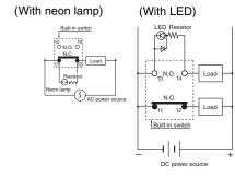
2) When the indication circuit is connected with load in parallel:
