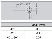
When V  $\leq$  0.2m/s, set the arm to perpendicular and set the arm rise angle to between 45° and 90°. If the dog rise angle is reduced, the maximum tolerable speed is increased. As a rule,  $\alpha = 45^{\circ}$  is optimum.
