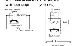
2. Lead wire type (only for types with LED) 1) When giving indication on N.O. side and N.C. side, operation is same as that in the case of the spring type. However, when load is connected to both N.O. side and N.C. side, indication can be given on both N.C. side and N.O. side. 2) When connecting load to N.C. side: When connecting switch is at free position, the indicator turns off, and when the switch operates, the indicator is lit. (Use the lamp holder, changing it direction by 180°.)
