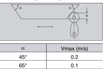
If overriding the dog, set the arm perpendicularly, so that  $\alpha$  =45°. If the dog angle is reduced, the tolerable speed is increased.
