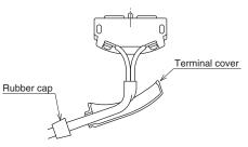
3. If using a VVF wire, bend the wire towards the unit, and once it has taken the proper shape, install the terminal cover. After installing the terminal cover, attach the rubber cap.
