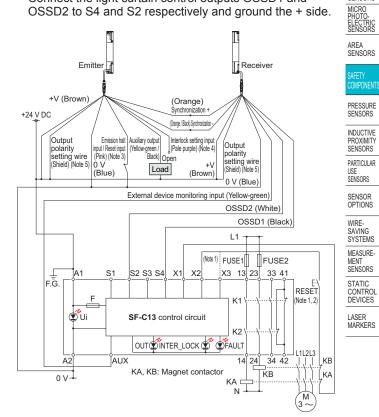
Notes: 1) The above diagram is when using manual reset. If automatic reset is used, disconnect the lead from X2 and connect it to X3. In this case, a reset (RESET) button is not needed.
