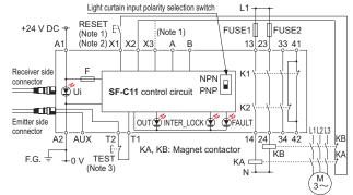
Notes: 1) The above diagram is when using manual reset. If automatic reset is used, disconnect the lead from X2 and connect it to X3. In this case, a reset (RESET) button is not needed.
