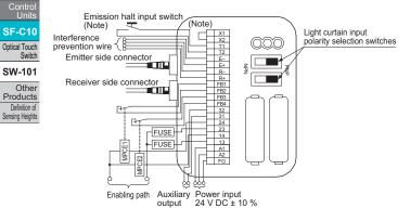
Note: The above diagram is when using manual reset. If automatic reset is used, connect a normal close-type pushbutton switch between T1 and T2 and leave between X1 and X2 open.
