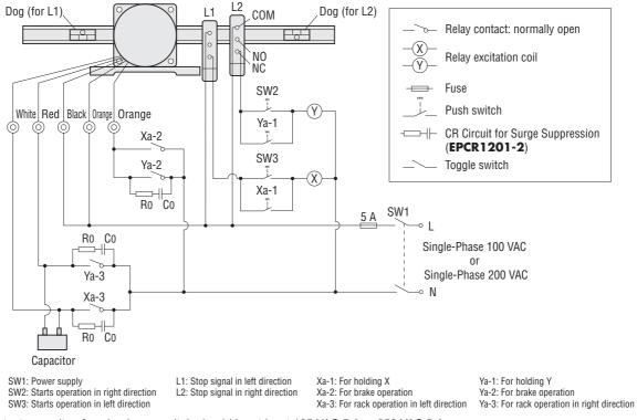
The contact capacity of each relay or switch should be at least 125 VAC 5 A or 250 VAC 5 A.
