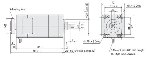
Dimensions 🛘 and 🔞 apply to a configuration with adjusting knob. For models without adjusting knob, the shaft and adjusting knob shown in \_\_\_\_ areas should be ignored.
