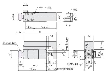
• The actuator comes with a motor lead wire/connector assembly (0.6 m). UL Style 3265, AWG24
