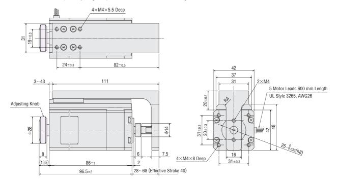
15 DRL42PB2G-04MG (With electromagnetic brake) DRL42PA2G-04MG (With electromagnetic brake)
