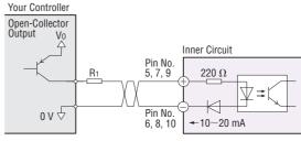
• Keep the input signal voltage Vo between 5 VDC and 24 VDC. When Vo is equal to 5 VDC, the external resistor R<sub>1</sub> is not necessary. When Vo is above 5 VDC, connect R<sub>1</sub> to keep the current between 10 mA and 20 mA
