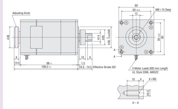
Dimension [9] applies to a configuration with adjusting knob. For models without adjusting knob, the shaft and adjusting knob shown in \_\_\_\_\_ area should be ignored.
