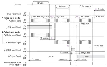
The shaded section indicates that the photocoupler is on
