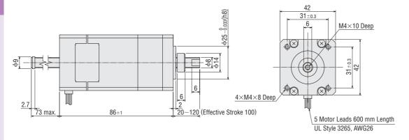
**BDRL42PB2-04MG** (With electromagnetic brake) **DRL42PA2-04MG** (With electromagnetic brake)
