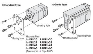
There are three ways of mounting an actuator to device.
