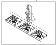
Driving a pump actuator device
