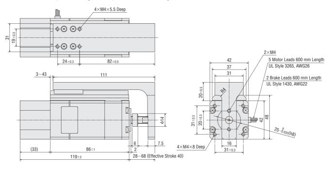
Dimension [4] applies to a configuration with adjusting knob. For models without adjusting knob, the shaft and adjusting knob shown in \_\_\_\_\_ areas should be ignored.
