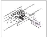
Adjusting a mirror positioning device
