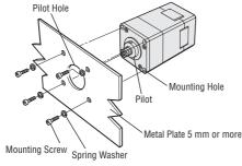
(The figure shows installation for standard type.)
