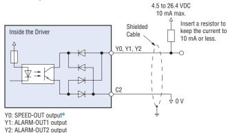
\*Supply a current of 5 mA or more to the SPEED-OUT output.
