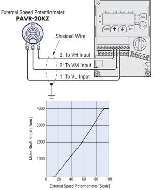
External Speed Potentiometer Scale – Speed Characteristics (Representative values)
