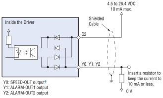
\*Supply a current of 5 mA or more to the SPEED-OUT output.
