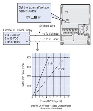
• The speed in the graph represents the speed of a motor alone. The gearhead output shaft speed of the combination type is calculated by dividing the graph speed by the gear ratio.
