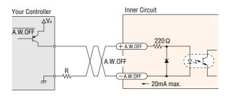
The external resistance R is not needed when  $V_{01}$  is 5V. When the voltage exceeds 5V, connect the external resistance R to keep input current at 20mA or less.
