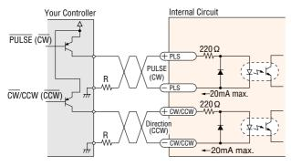
The characters indicate signals under the 1-pulse input mode, while the characters in parenthesis indicate signals under the 2-pulse input mode. The external resistance R is not needed when  $V_0$  is 5V. When the voltage exceeds 5V, connect the external resistance R to keep input current at 20mA or less.
