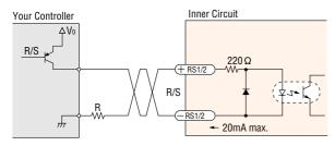
The external resistance R is not needed when  $V_0$  is 5V. When the voltage exceeds 5V, connect the external resistance R to keep input current at 20mA or less
