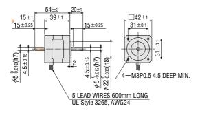
\* 15±0.25 indicates the length of milling on motor shaft.
