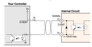
Keep the voltage between 5V and 24V and current at 10mA or less.
