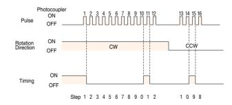
When used as indicated in the sample connection, the signal is in the "photocoupler ON" state at STEP 0.
