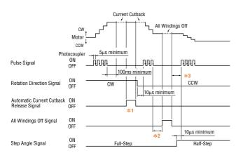
When the signal is in the "photocoupler ON" state, the "Automatic Current Cutback" function is deactivated. Always set it in the "photocoupler  $\ensuremath{\mathsf{OFF}}\xspace"$  state when the pulse signal is stopped.
