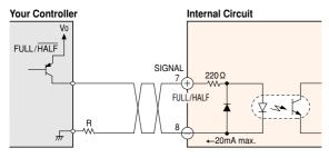
The external resistance R is not needed when  $V_0$  is 5V. When the voltage exceeds 5V, connect the external resistance R to keep input current at 20mA or less.
