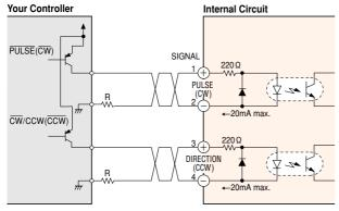
The characters indicate signals under the 1-pulse input mode, while the characters in parenthesis indicate signals under the 2-pulse input mode. The external resistance R is not needed when  $V_0$  is 5V. When the voltage exceeds 5V, connect the external resistance R to keep input current at 20mA or less.
