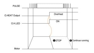
The "Automatic Current Off" function select switch can be used to determine how the "O.HEAT" signal affects the motor's operation.
