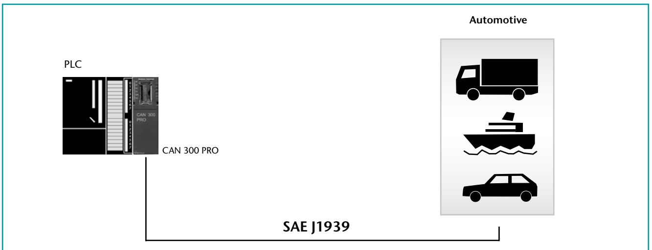
Application Example CAN 300 PRO SAE J1939 Protocol
