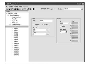
The CAN modules contain acceptance masks. These masks can be used to enable or disable various telegram IDs for reception. Express masks filter high-priority CAN telegrams so that they can be forwarded directly to the PLC.
